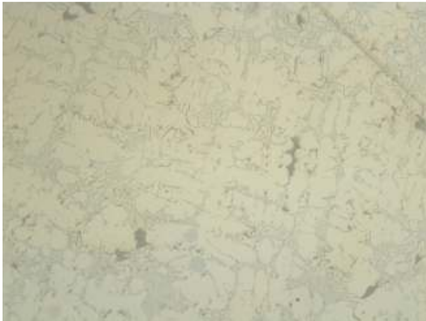
Photo 8 Chill cast showing porosity. Showing fine graphite (dark areas) in a single alpha phase (light areas) with porosity showing black. Magnification approximately X200
