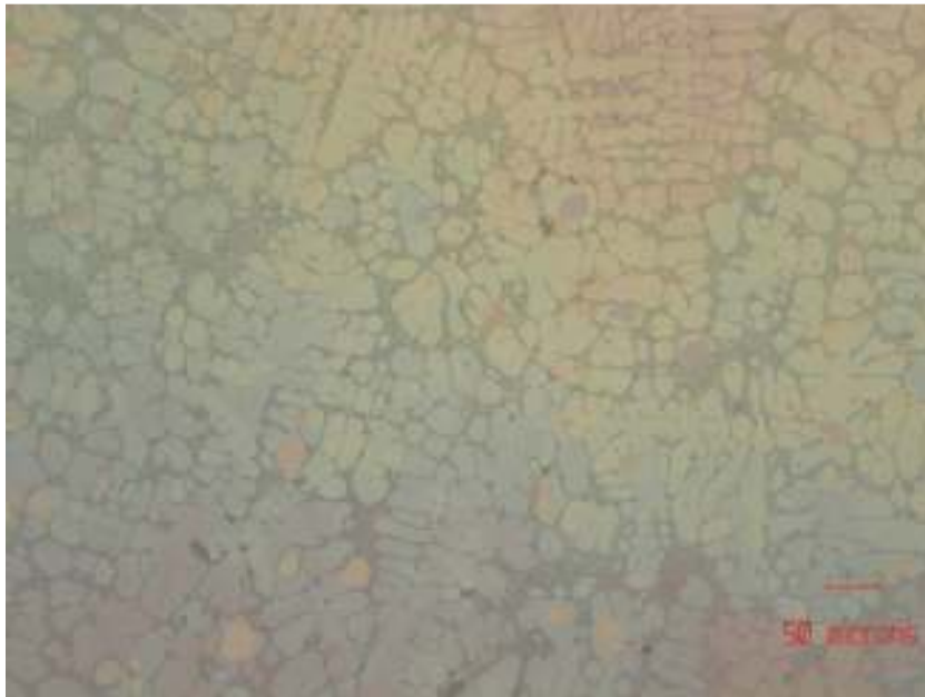
Photo 3 Centrifugal casting. Showing fine graphite (dark areas) in a single alpha phase Magnification approximately X100
