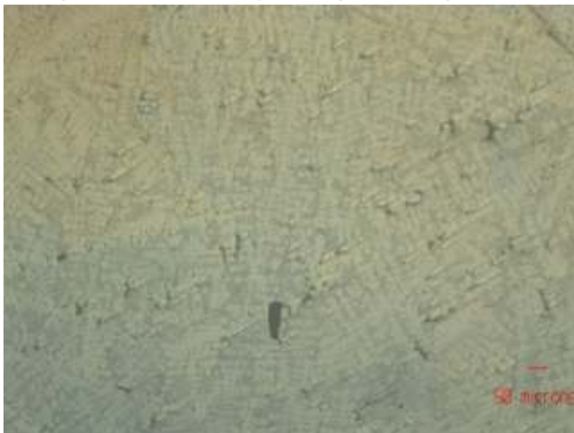
Photo 6 Chill cast showing porosity. Showing fine graphite (dark areas) in a single alpha phase (light areas) with porosity showing black. Magnification approximately X50
