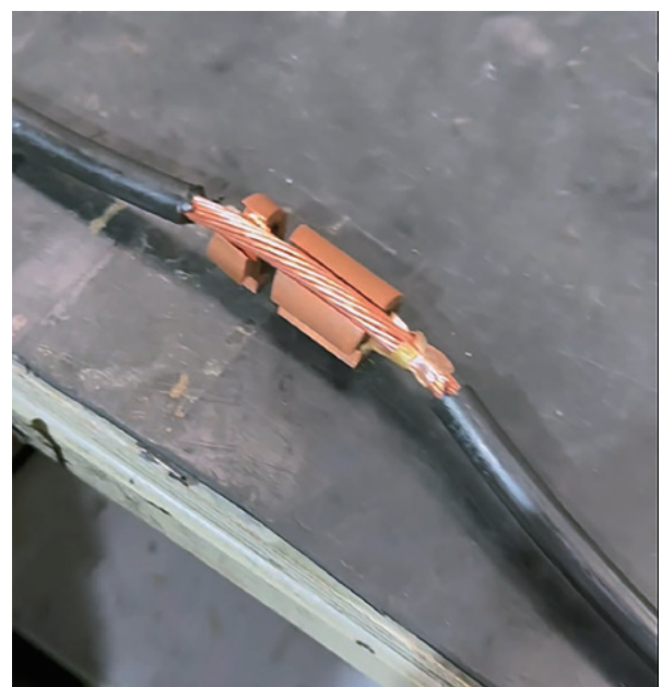
Anode Connector Installation Illustration
