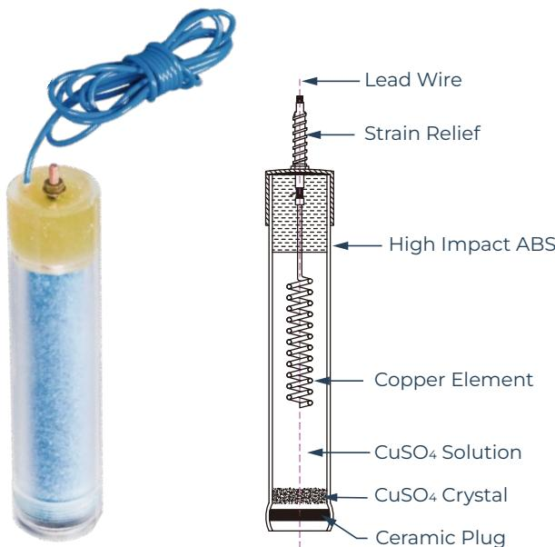
■ Bagged Copper/Copper Sulphate Reference Electrode
